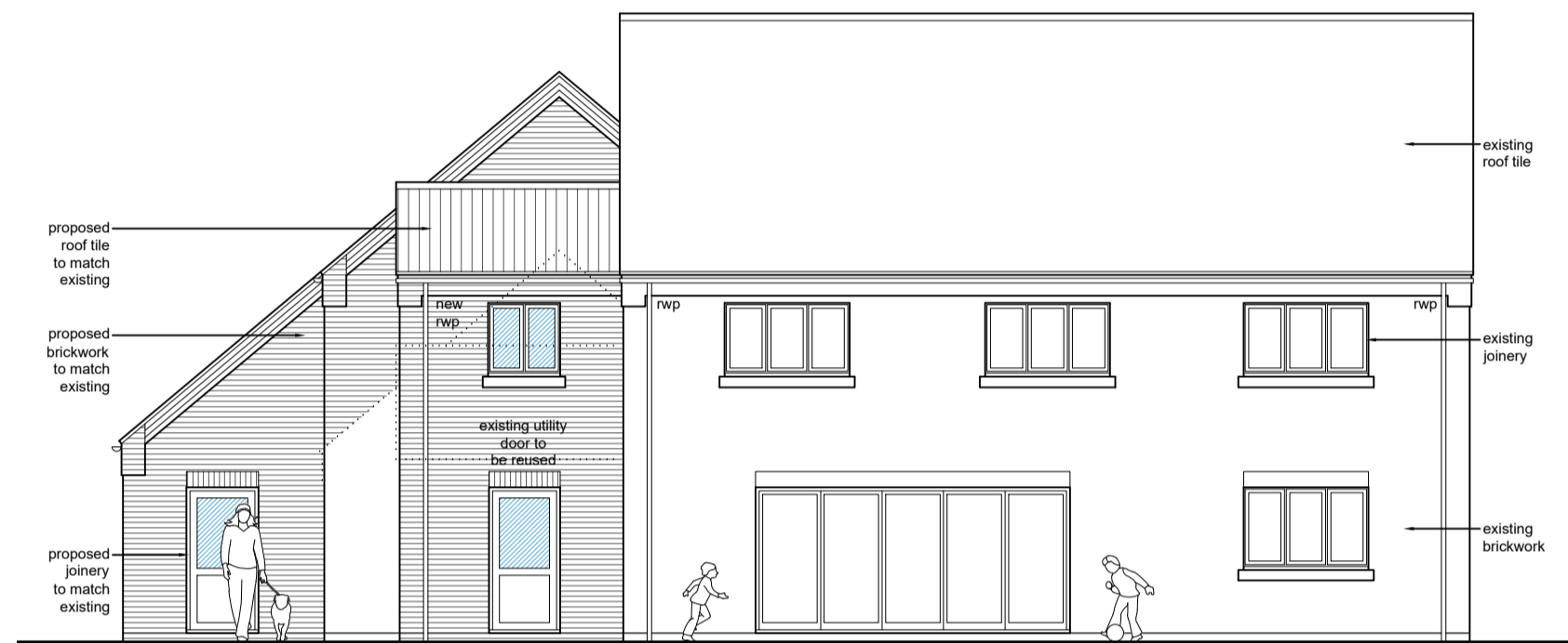
Rear Elevation (S) Scale: 1:100
