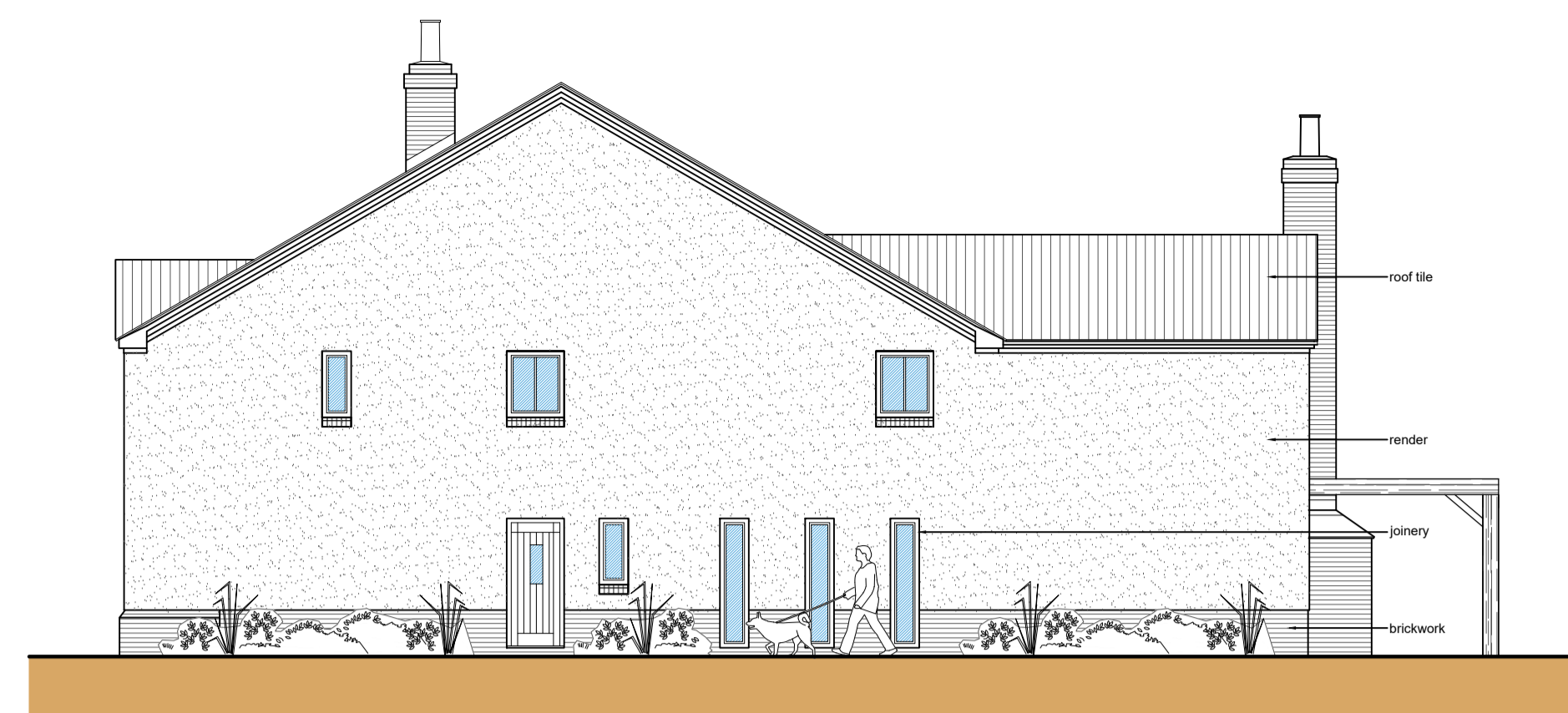
Side Elevation (NE) Scale: 1:100 metres
