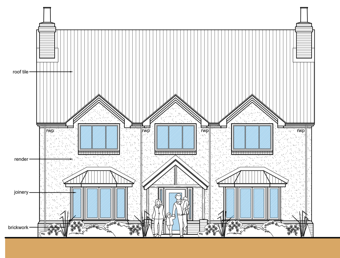
Front Elevation (SE) Scale: 1:100 metres
